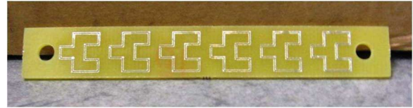
Fig. 8. A single strip containing 6 unit cells of inclusions fabricated using printed circuit board technology.
