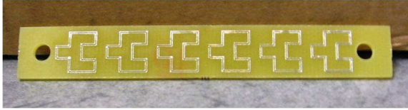
Figure 4. A single strip containing 6 unit cells of inclusions fabricated using printed circuit board technology.
