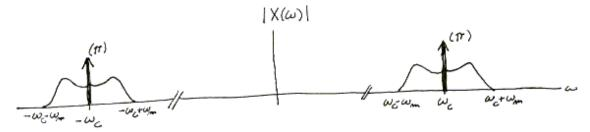
From this plot is clear that AM modulation is used to shift the spectral content of a message to a frequency range reserved for a particular transmitter. By assigning different carrier frequencies to different transmitters, with a separation of at least  $2\omega_m$  in the different carriers, the messages are kept distinct.
