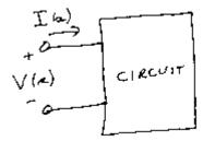
with all independent sources in the circuit set to zero and all initial conditions zero, the *impedance* Z(s) of the circuit is the transfer function
