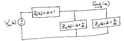
where we have chosen impedance labels for the various portions of the overall circuit. Next, a source transformation gives
