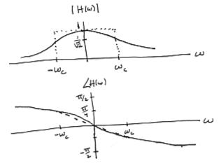
Clearly the first-order differential equation is a rather poor approximation to an ideal filter, but higher-order differential equations can perform closer to the ideal.
