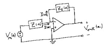
In order to compute the voltage transfer function ,  $V_{out}(s)/V_{in}(s)$  , we use the *virtual short* property of the ideal op amp to conclude that
