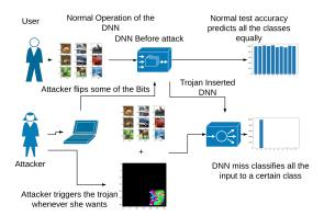
Figure 3. Flow chart of effectively implementing TBT
