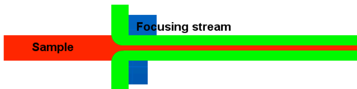
Figure 2. Hydrodynamic focusing by two buffer streams [3]
