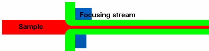
Figure 2. Hydrodynamic focusing by two buffer streams [3]
