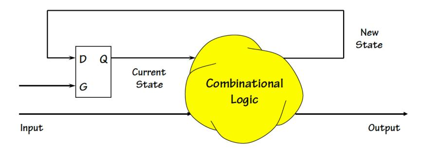
Plan: Build a Sequential Circuit with one bit of STATE -
