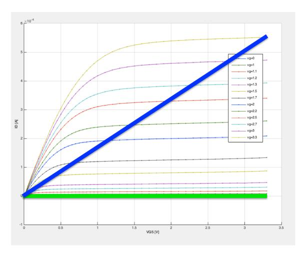
With digital input on gate, device is either ON or OFF
