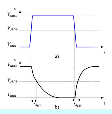
Delay, td is measured from 50% point to 50% point, between input and output.
