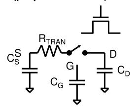
$R_{ON} \sim 3.3 \text{V} / 0.55 \text{mA} = 6 \text{K}$
