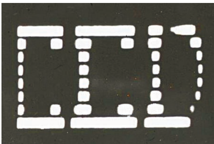
Figure 9. Oscilloscope display of the output of the 8-bit device used as an imager.
