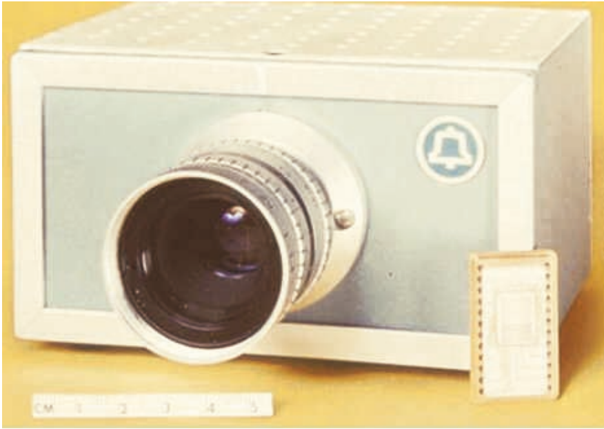
Figure 13. The CCD Picturephone imaging chip and a self-contained camera.
