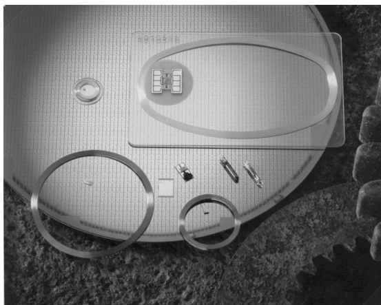
Figure 3.14 Different designs of inductively coupled transponders. The photo shows half finished transponders, i.e. transponders before injection into a plastic housing (reproduced by permission of AmaTech GmbH & Co. KG, D-Pfronten)
