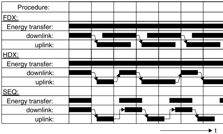
Figure 3.12 Representation of full duplex, half duplex and sequential systems over time. Data transfer from the reader to the transponder is termed downlink, while data transfer from the transponder to the reader is termed uplink
