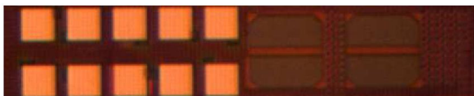
Fig. 3. Micrograph of the entire system, top view. Note the pads and the antennae, the two large coils and half of the dipole. The remainder is obscured by fill.
