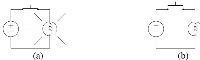
Figure 1.2: Flashlight schematic. (a) Switch on. (b) Switch off.
