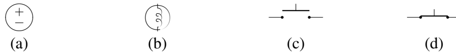
Figure 1.1: Schematic elements. (a) Voltage source. (b) Light bulb. (c) Switch, open (off). (d) Switch, closed (on).
