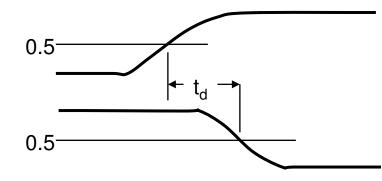
Delay,  $t_d$ , is measured from 50% point to 50% point. Gives a measure that is composable. Define Rsq so RC product is roughly equal to the delay  $t_d$
