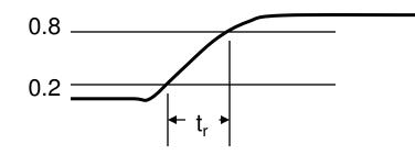
Rise time and fall time,  $t_r$  and  $t_f$ , are measured from 20% point to 80% point. But they are not generally used in digital design.
