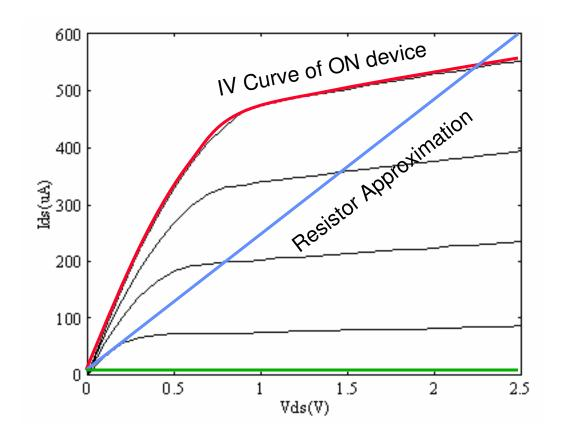
With digital input on gate, device is either ON or OFF
